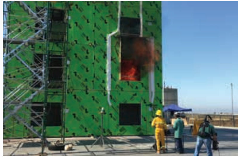
Photo 2: After a series of simulated earthquakes, the second and sixth floor were set on fire to analyze the full effects of a natural disaster.
