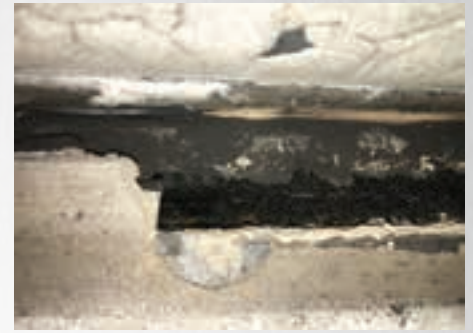
Photo 5: HOT ROD on the fire side. The intumescent material expands under fire and seals against the ceiling which prevents any smoke from passing to the non-fire side.
