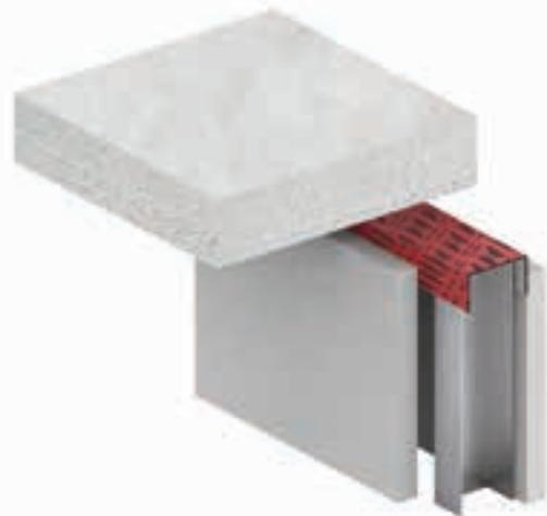
SpecSeal® TTG makes short work of construction joints in gypsum board construction. TTG eliminates the need for firestop sealants or sprays. TTG is easily cut to length with scissors or a sharp knife, installing quickly with no waste. It's red in color for easy identification and inspection.
